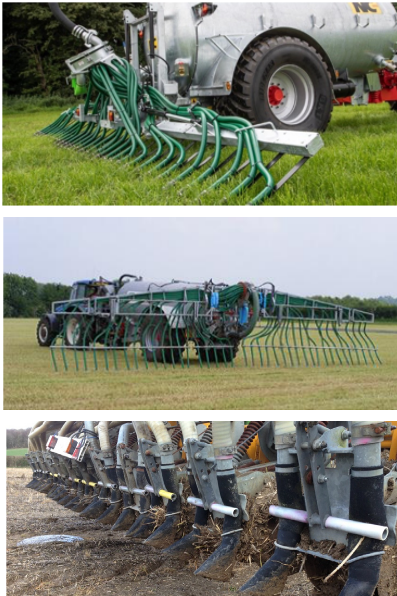
Figure 9. Low Emission Slurry Spreading Equipment: Top - a trailing shoe system; middle - a trailing hose system; bottom - a shallow injection system.
