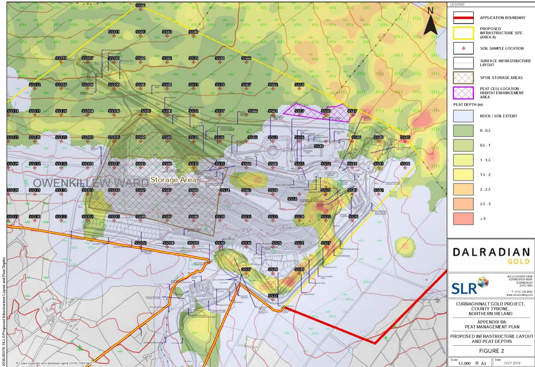
Figure 8.1: Copy of PMP Figure 2 showing the proposed habitat enhancement area (pink cross-hatching) and peat storage area within the DSF footprint (brown cross-hatching).
