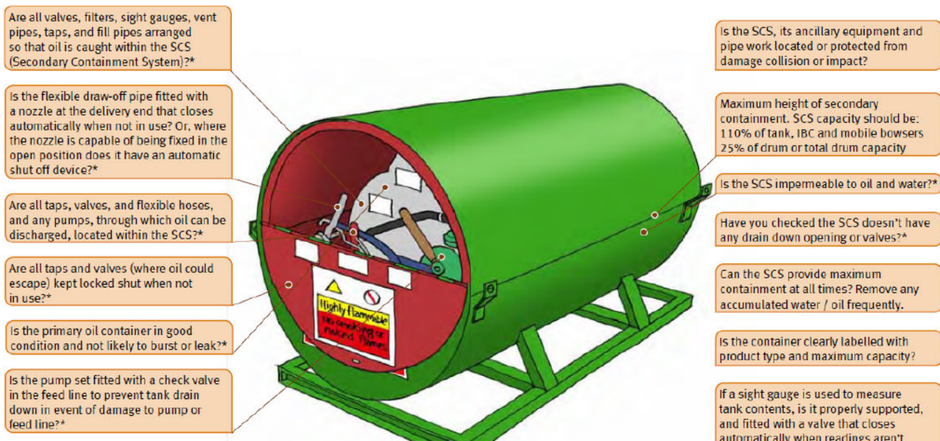
Figure 8 - Illustration of oil storage with a secondary containment system
