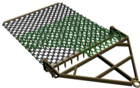
Figure: A diagram representing a Newhaven scallop dredge
