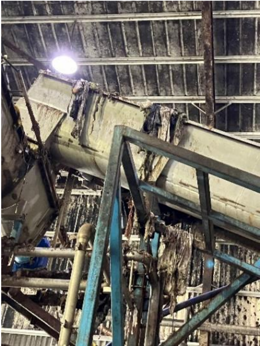
Photo 8 Waste falling out of transfer machinery
