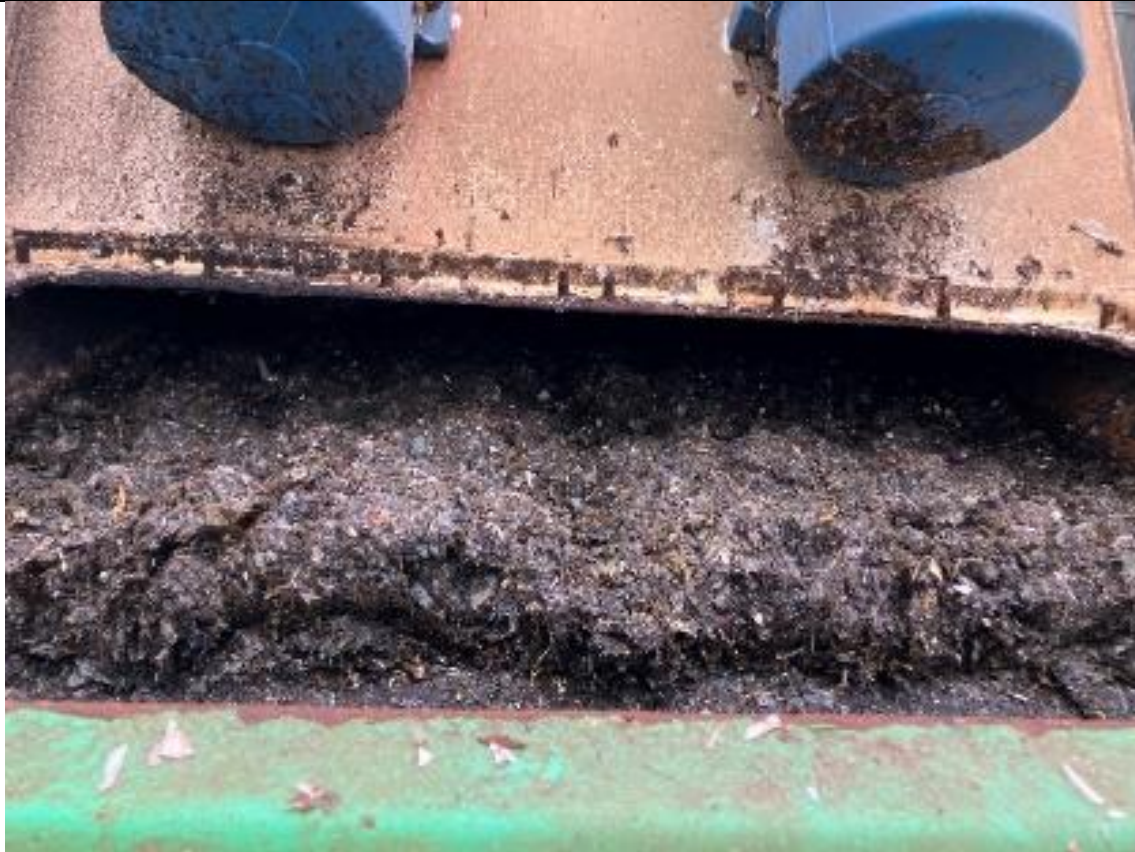
Photo 18 Digestate screener waste
