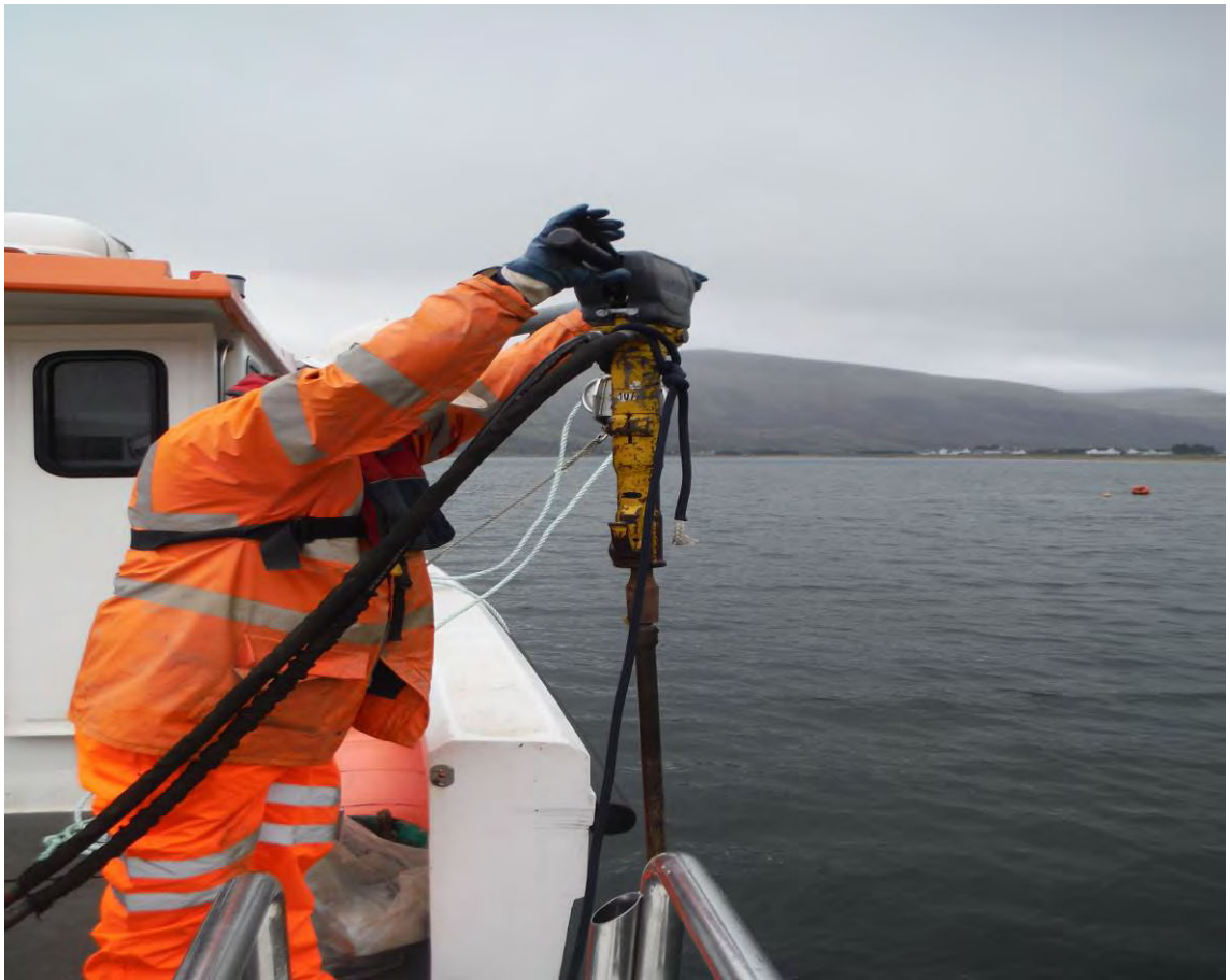
Dual Tube Sampler Driven into Sea Bed
