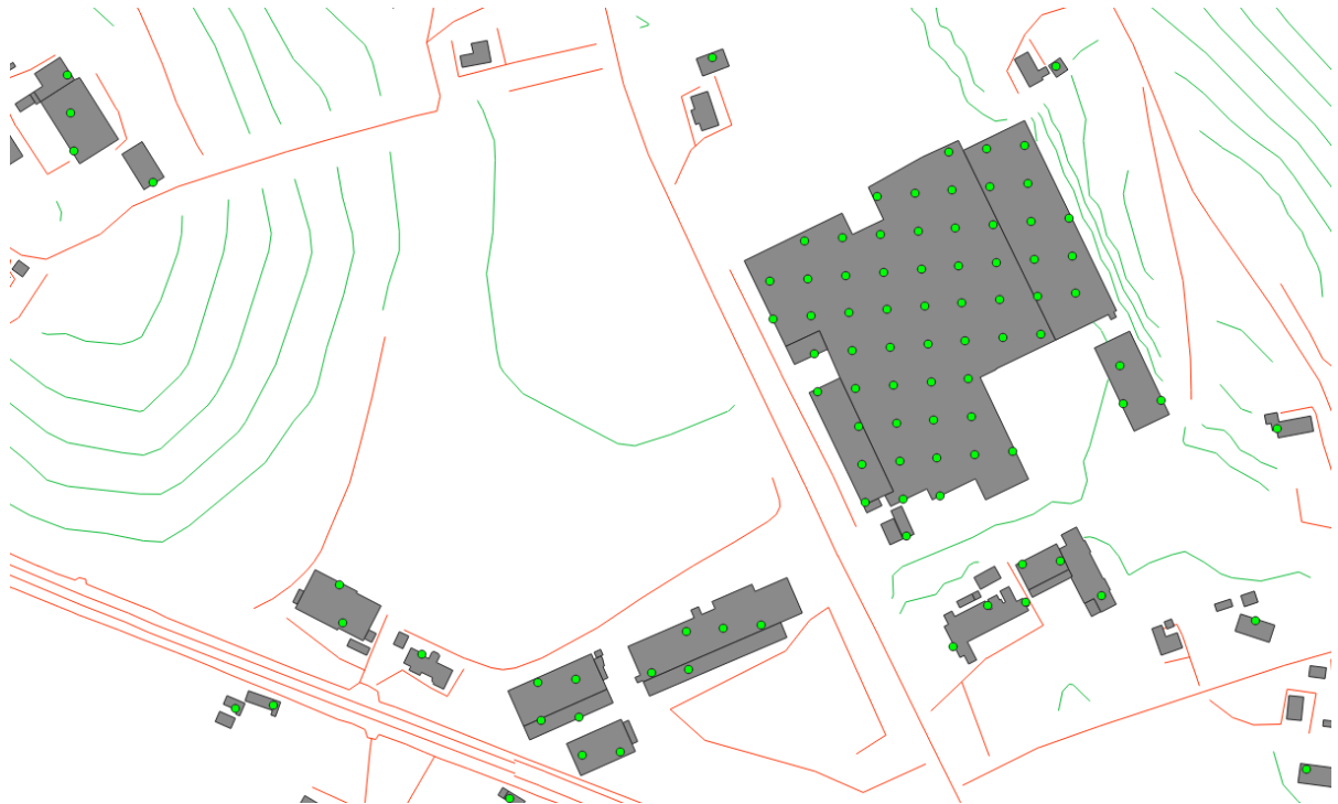
Figure 8: Example of Building Interaction Against Equal Height Contours, Breaklines and Spot Heights in GIS
