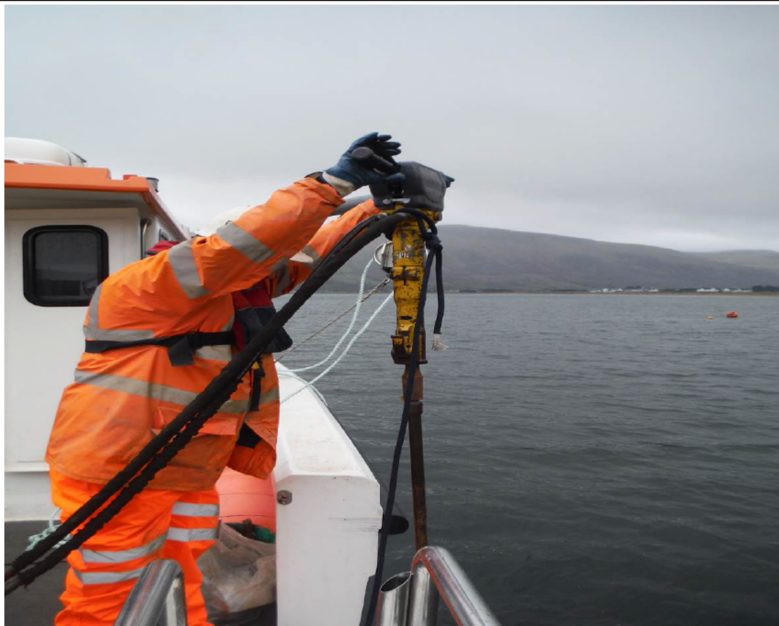
Dual Tube Sampler Driven into Sea Bed
