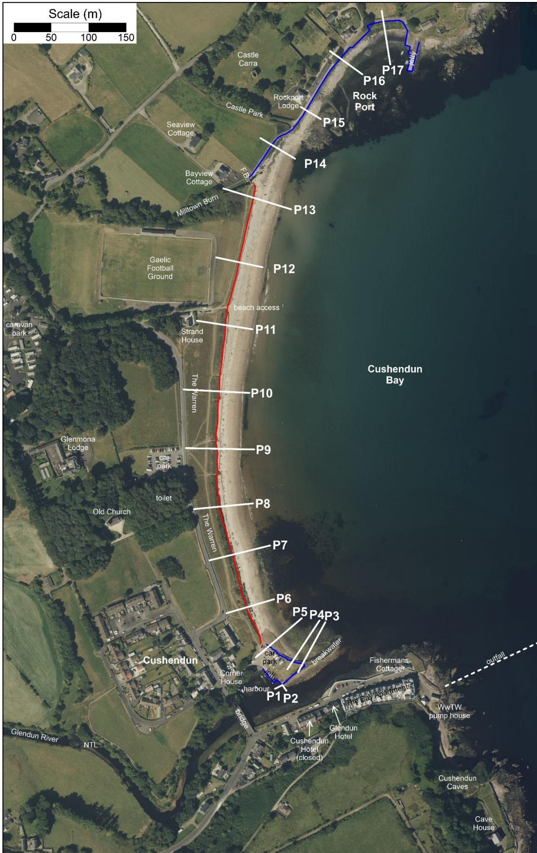
Figure A2.8 Aerial photograph flown c. July 2022, overlaid with the position of the dune toe (red line), sea defences (blue line) and cross-shore profiles (white lines) surveyed in May 2024. Source: Bing
