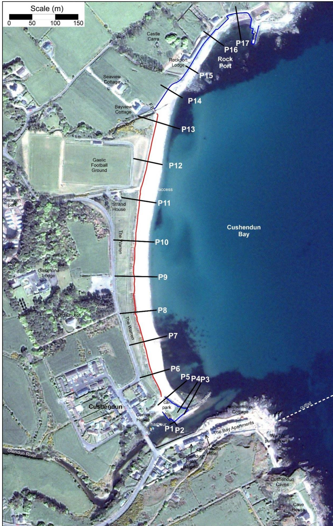
Figure A2.6 Aerial photo flown 13/05/2001, overlaid with the position of the dune toe (red line), sea defences (blue line) and cross-shore profiles (black lines) surveyed in May 2024. Source: Google Earth
