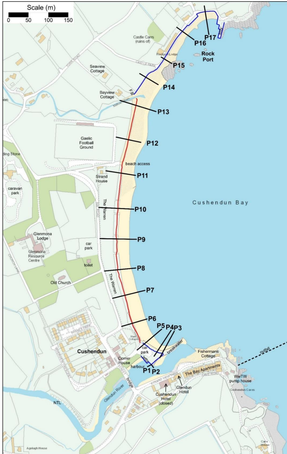
Figure 14. Locations of profiles used for RTK-GNSS topographic monitoring in this study. The red line indicates the dune toe and the blue line indicates the seaward limit of vegetation (usually the top of defences or seaward side of paths or roads) surveyed in May 2024
