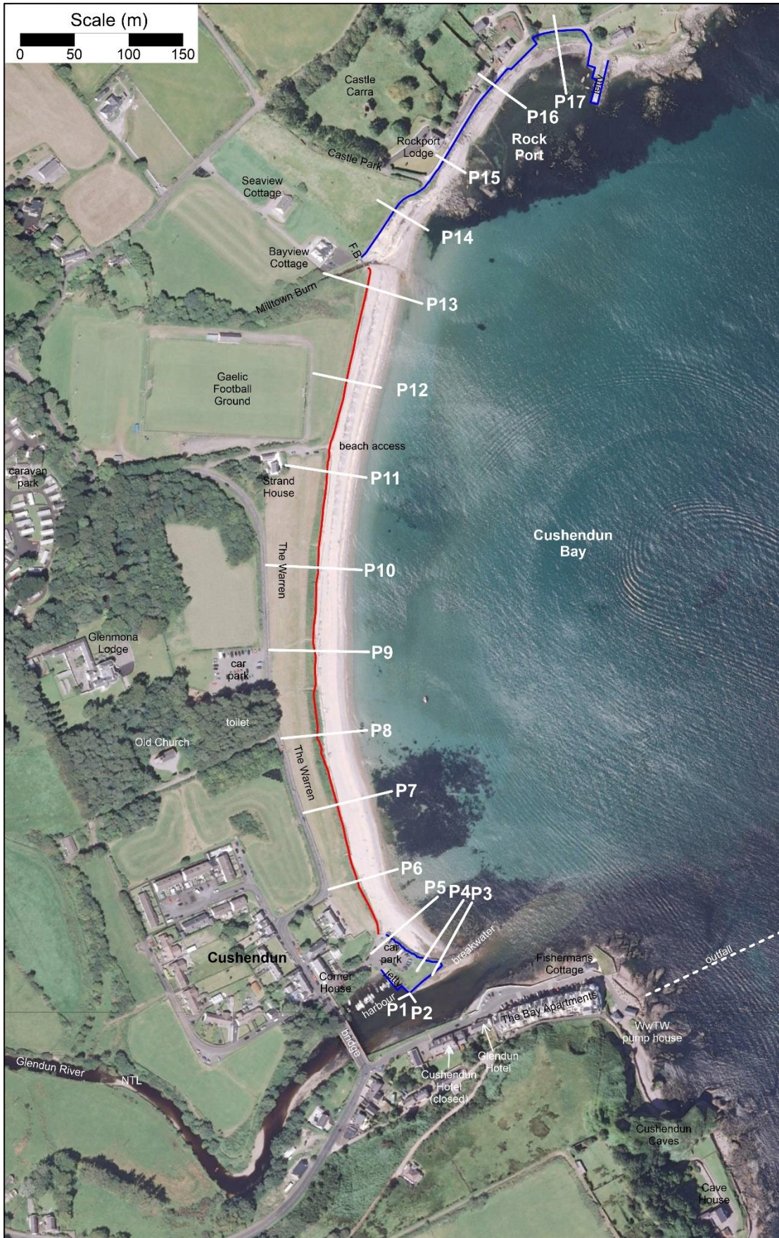
Figure A2.7 Aerial photo flown 24/07/2011, overlaid with the position of the dune toe (red line), sea defences (blue line) and cross-shore profiles (white lines) surveyed in May 2024. Source: Google Earth
