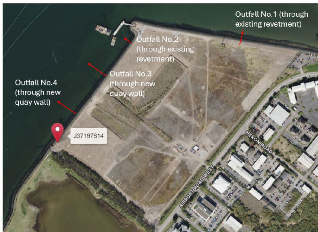
Figure 2.1 - Location of 4 no. outfalls – two of which are through quay wall, and the other two through the revetment
