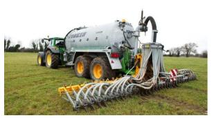
Figure 4 shallow injection equipment
