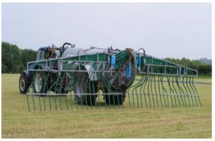
Figure 2a Tanker with trailing hose
