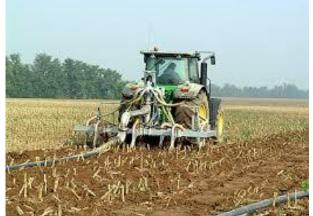
Figure 5 Deep slurry Injection equipment
