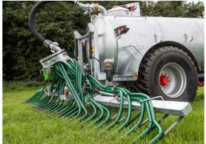
Figure 3b Trailing shoe slurry application.
