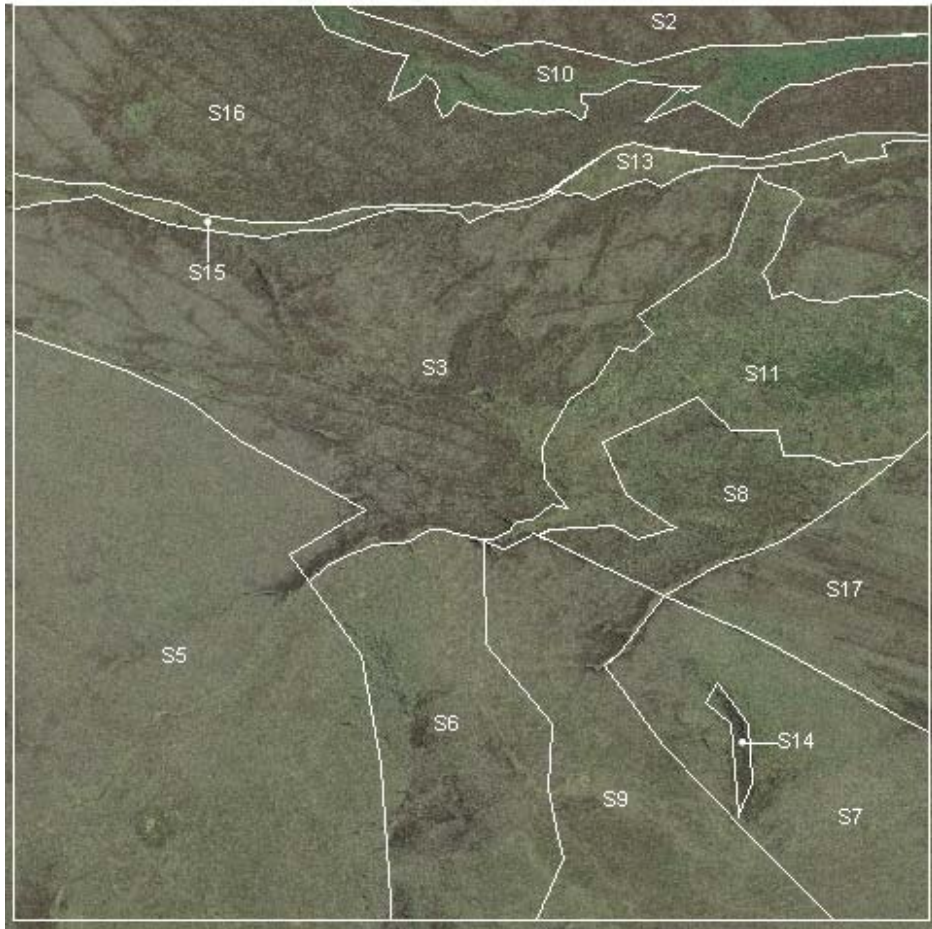
Fig. 6.3.1 Vegetation boundaries mapped using field observation, the aerial photograph (wavy boundaries) and about 20-30 key GPS points (straight/angular boundaries).
