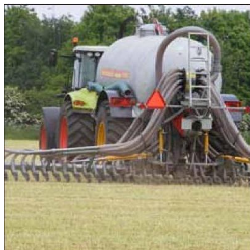
Photo 3 - Trailing shoe spreader
